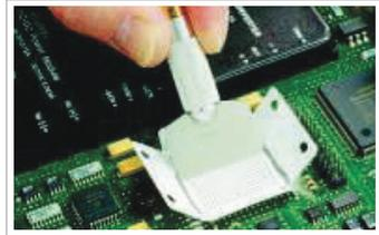
**Step 5.** Remove the stencil and save for another reuse or dispose
